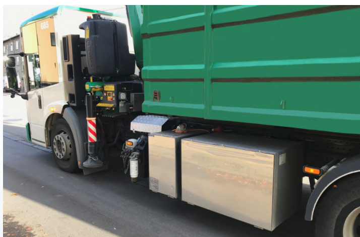
Typical installation of Banke CM36 E-PTO with power box on the left and battery box to the right
